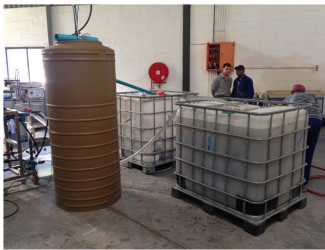
Photograph 2: Shows the 1m 3 Raw Effluent Feed Tank (right foreground), the 0.75m 3 Clarifying Tank (left foreground), and Sludge Collection Vessel (at the back).
