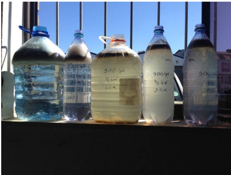
Photograph 8: Shows the Electro-Coagulation Sample No. 1 after a clarification stand time of 5 minutes against sample of the Raw Effluent Feed-Stock. The reduction in turbidity and improvement in clarity can clearly be seen.
