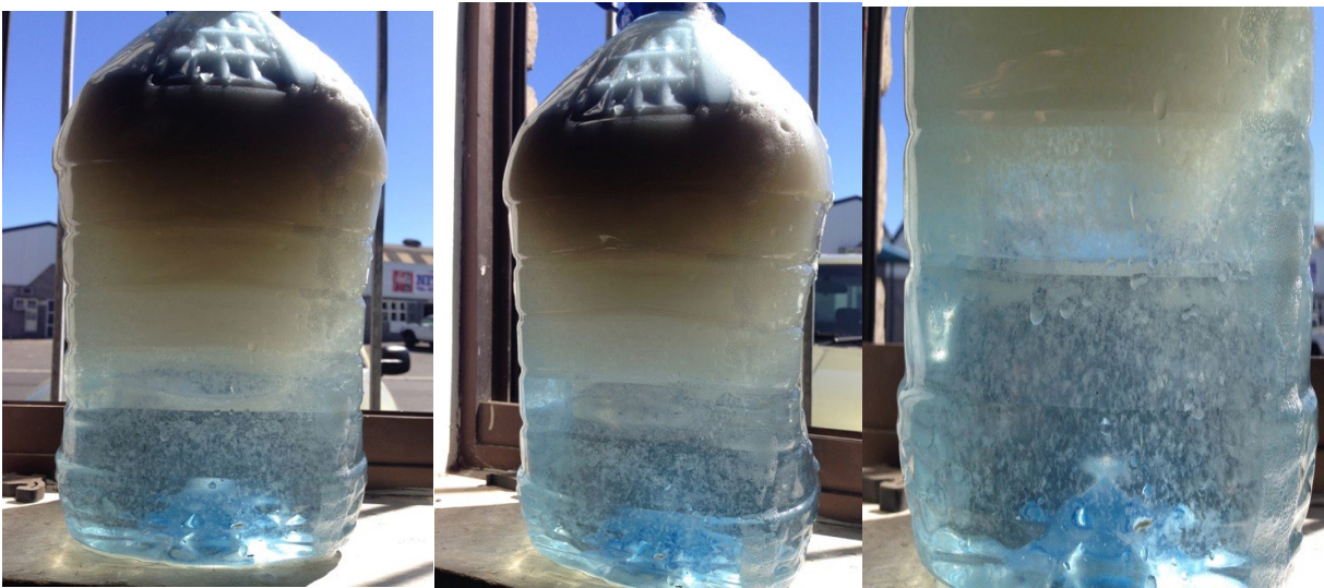
Photograph 5, 6 & 7: Shows the Electro-Coagulation Sample No.1 under Clarification Stand. The first picture was taken at 90 seconds from the time of placing the sample to stand, and the subsequent pictures at 30 second intervals thereafter/
