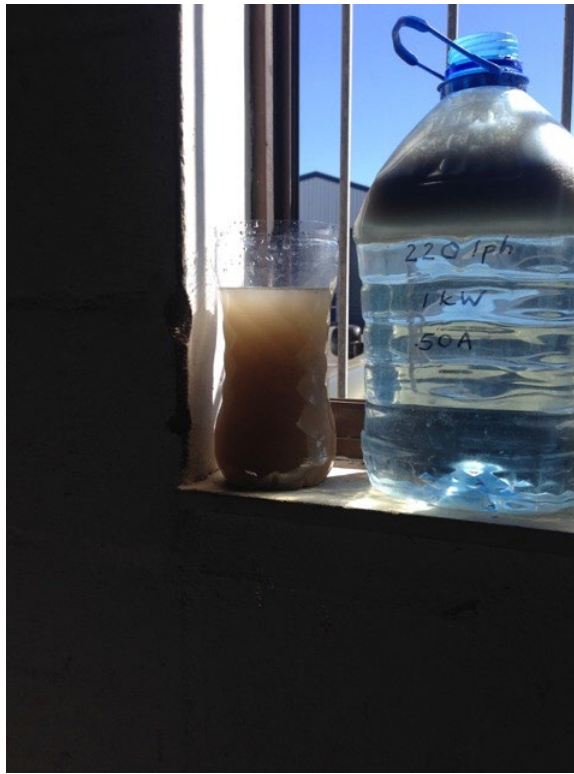
Photograph 8: Shows the Electro-Coagulation Sample No. 1 after a clarification stand time of 5 minutes against sample of the Raw Effluent Feed-Stock. The reduction in turbidity and improvement in clarity can clearly be seen.
